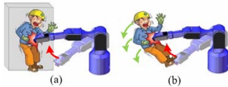
Fig. 16. Types of collision: (a) constrained impact and (b) unconstrained impact.
