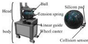
Fig. 15. Experimental setup to represent human head and body for collision experiment.
